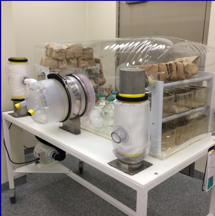
Isolator Housing to maintain Germ Free and Gnotobiotic mice.
