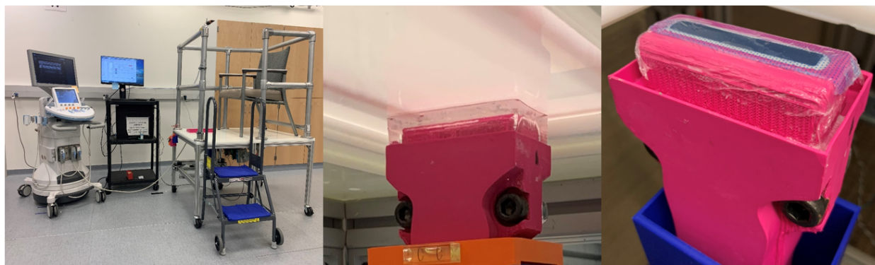
Figure 3: Left: setup for volumetric ultrasound scans. Subjects ascend the stairs and either sit in the chair or stand placing equal weight in the scanning area and the non-scanning area. The computer hosts the MATLAB-based control program and the system uses an Aixplorer commercial ultrasound machine.
