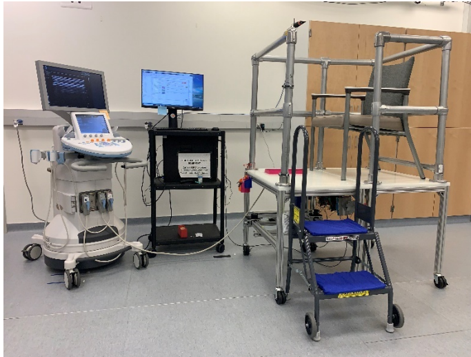
Figure 1: The final constructed scanner including both mobile halves secured together, a set of stairs with handles, motors, linear actuators, and DIN rail mounted electrical system, HDPE plate and water bath, and a chair for the subject to sit on during unweighted data collections.
